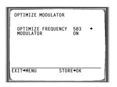
Select line 'OPTIMIZE FREQUENCY' using  $P \uparrow +$  or  $P \downarrow -$ . Enter the new modulator frequency with the number buttons 0-9.
